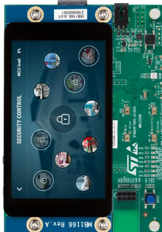
32F769IDISCO STM32F769 800x480 WVGA LCD 128 Mbits SDRAM 512 Mbit QSPI Flash Arduino Uno
