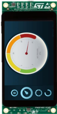
32F469IDISCO STM32F469 800x480 WVGA LCD 128 Mbits SDRAM 128 Mbit QSPI Flash Arduino Uno
