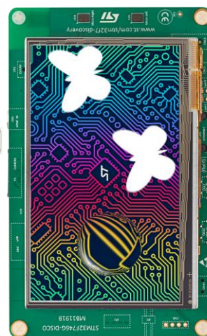
32F750GDISCO STM32F750 480x272 WQVGA LCD 64 Mbits SDRAM 128 Mbit QSPI Flash Arduino Uno
